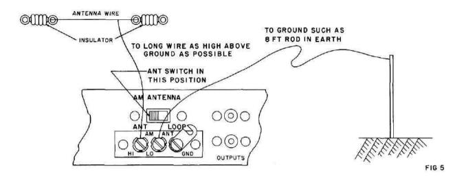
An outside AM antenna is a wire as long as practical, mounted as high as possible above the ground, at right angles to power lines. The lead in should be carefully positioned away from all A. C, lines.
