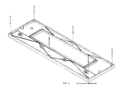
The tuner panel is now ready to be attached to the cabinet. The six threaded-rods are inserted through the two 5/32 inch and the four 3/16 inch holes in the cabinet panel. Secure the tuner panel to the cabinet panel by installing on the rods the 6/32 "KEP" nuts supplied in the parts bag. Bring the nuts up tight with a wrench or nut driver.
